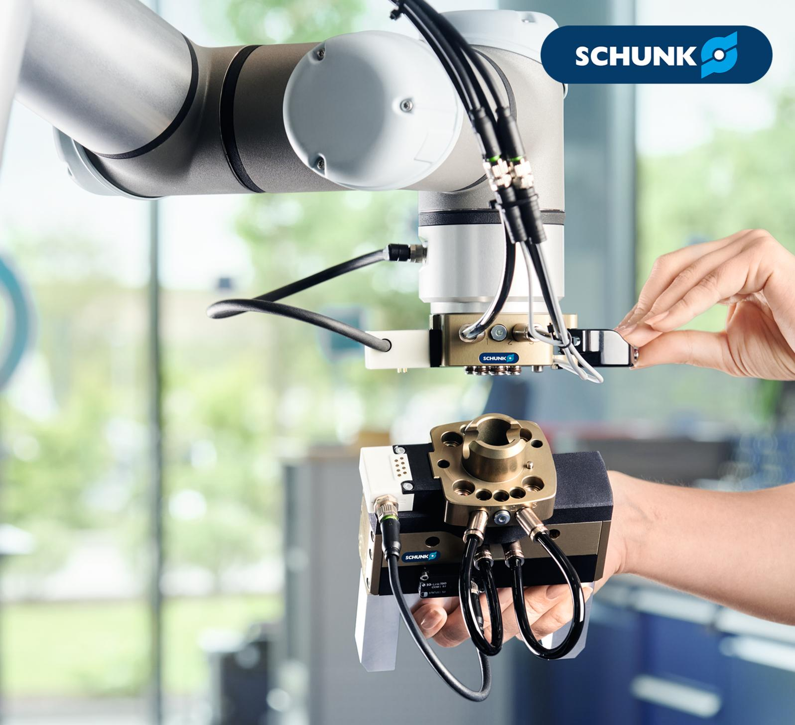
The image shows a robotic arm with a SCHUNK CMS manual changeover system. A person's hand is shown adjusting a component on the robot's gripper. Below, another hand holds a separate component of the system, which is a black and brass-colored metal block with various ports and a central opening. The background is a blurred industrial setting with large windows.
